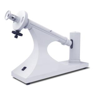
Easy-to-use manual polarimeter, measuring range from -180 to +180 degrees. The instrument is suitable for measuring the optical rotation of the optically active substances, accuracy: 0.05 degrees.
